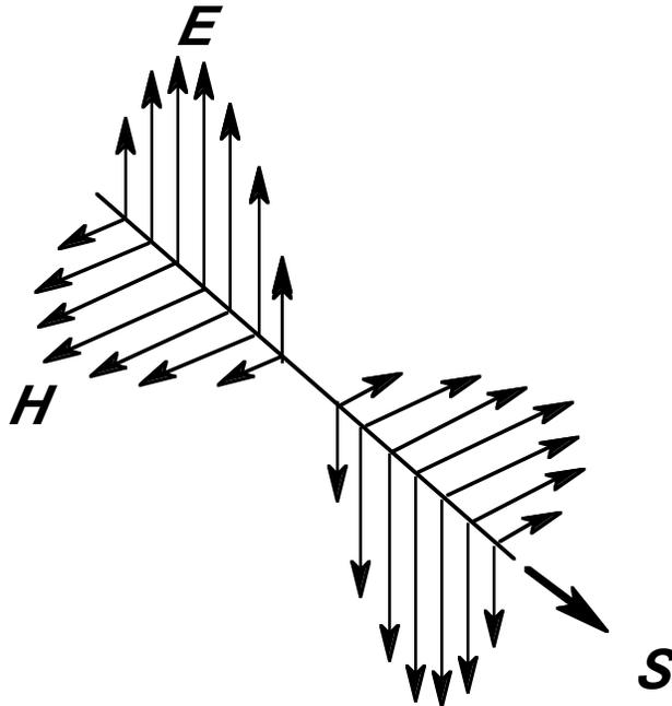
The vector  $S$  is the Poynting Vector. Its magnitude is the amount of energy carried by the wave and its direction is the direction of propagation of the wave.
