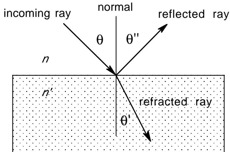
The law of reflection is easy, the angle of incidence equals the angle of reflection, or
