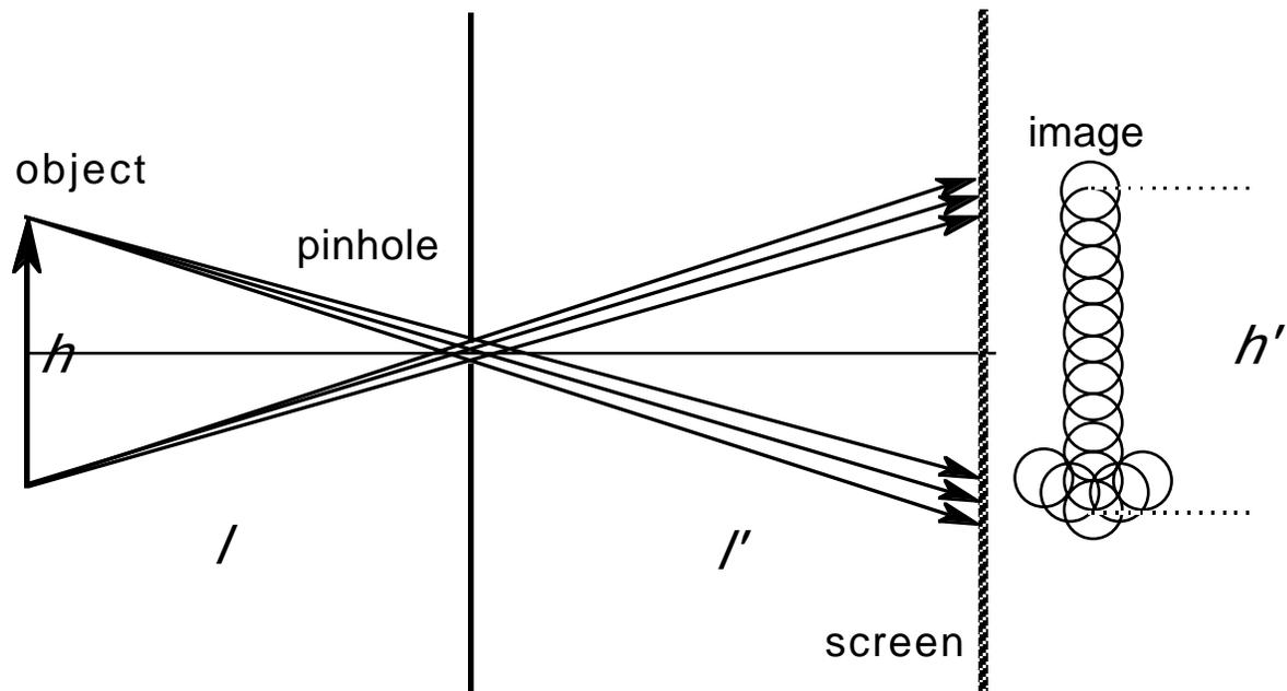
Each point on the object is imaged as a small circle, and these circles combine to form a somewhat fuzzy image of the object. The smaller the pinhole, the sharper--and dimmer--the image. The size of object and image are related to the pinhole position by the equation
