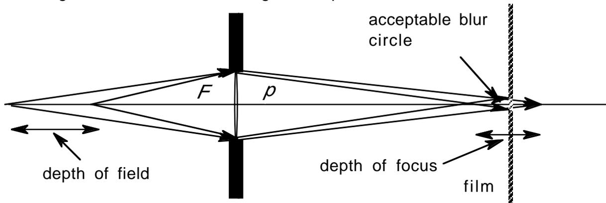
The distance through which a point source may be moved without its image exceeding the acceptable blur circle in the film plane is called the depth of field. The conjugate distance around the film plane is called the depth of focus.
