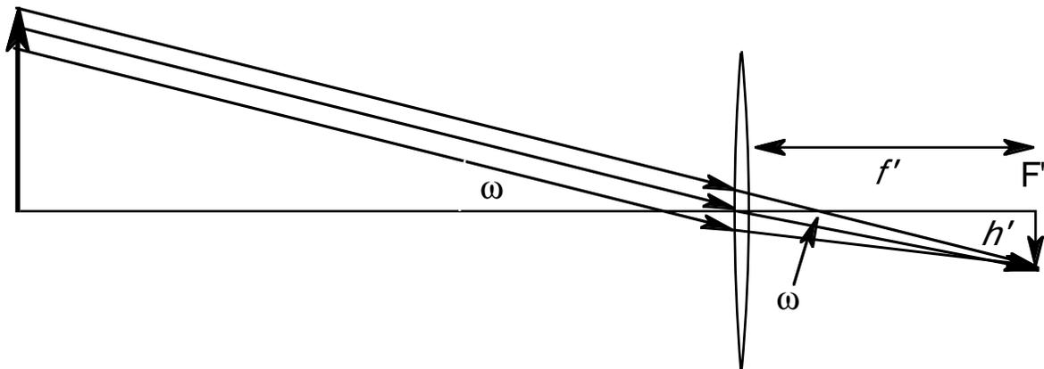
Suppose a remote object subtends angle  $\omega$  in object space in front of a thin lens. Its image is formed at the secondary focal point a distance  $f'$  behind the lens. The height of the image may be determined from the similar triangle in image space to be
