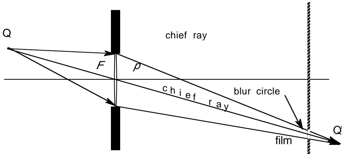
The diagram above shows how the aperture determines the degree of blur of an out-of-focus image. Clearly, the blur circle radius is proportional to the aperture radius. In any optical system there is an acceptable degree of blur. Blur circles below a certain size are recognized as points. The distance through which an object can move without producing an image that is unacceptably blurred is called depth of field.
