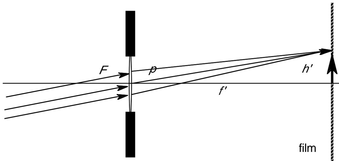
The camera shown above forms the image of a remote object. The illuminance  $E$  of the image on the film equals the amount of light (luminous flux) which reaches the image divided by the area of the image. Clearly the amount of light that can get into the camera is proportional to the area of the aperture around the lens which is proportional to the square of the radius of that aperture,  $\rho$ , or in equation form
