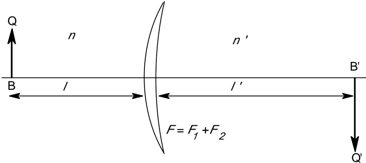
These last two equations tell us that the thin lens acts like a single optical entity with power  $F = F_1 + F_2$  which obeys the fundamental paraxial equation
