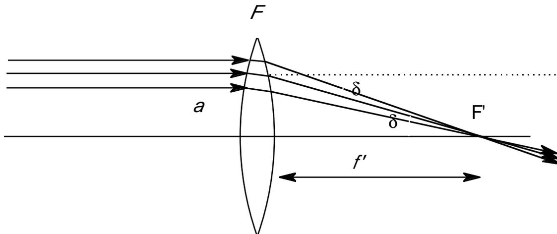
Consider a parallel bundle of rays striking a lens of power  $F$  a distance  $a$  from the optical axis. Rays converge to the secondary focal point. The ray bundle is rotated through an angle  $\delta$  where  $\delta = -a/f' = -aF$ . To get the prismatic deviation, remember that prism power  $\Delta$  is one hundred times the angle of deviation in radians so
