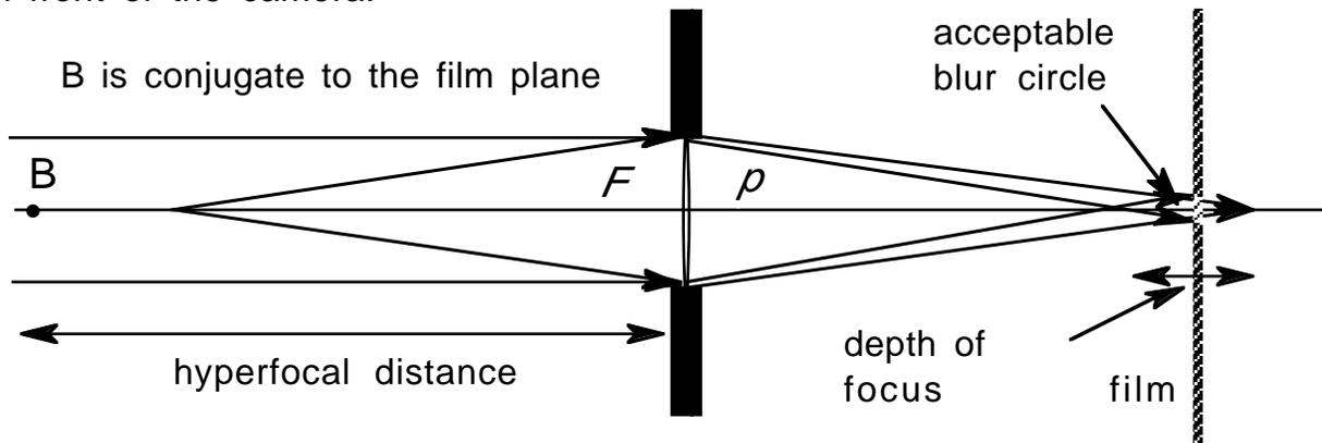
When a camera is focused for the hyperfocal distance, its linear depth of field is infinite. Simple fixed focus cameras are set for the hyperfocal distance. The hyperfocal distance for the eye is about six meters (20 ft) which is why optometrist's eye charts are 6 meters from patients in a typical examination room.
