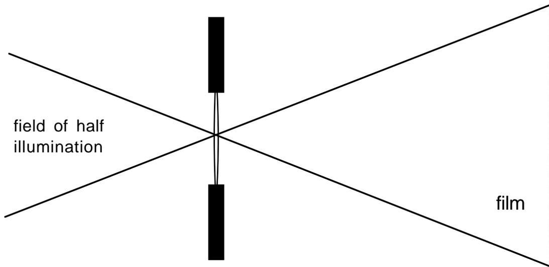
This is called the field of half illumination because the illumination of an image at the edge of the film is half what it would be if it were formed at the center of the film.
