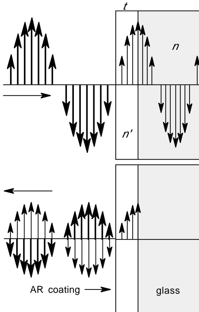
The figures above shows how an AR coating works. The top figure shows light incident on a lens and its coating. The bottom diagram shows light reflected from the air-coating interface and the coating-glass interface. The coating and its thickness are chosen so the two wavefronts have the same amplitude and are exactly out of phase so the cancel when combined.
