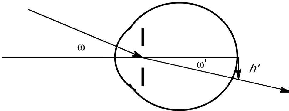
In terms of the diagram above, this says that  $h' \propto \omega' \propto \omega$ . So if we want the ratio of two image heights, all we need calculate is the ratio of the angles the chief ray makes with the optical axis after leaving the lens (or other optical device) placed before the eye to the angle it would have made without the lens. That, it turns out, is a property of the lens independent of the eye.
