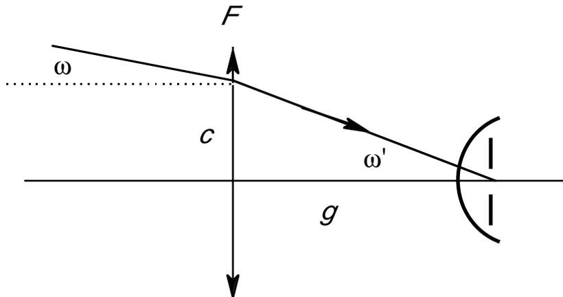
From Prentice's rule, the deviation  $\delta$  of the rays is  $\delta = Fc$ . But  $\delta = \omega' - \omega$  so  $\omega' - \omega = cF$ . The spectacle magnification is  $SM = \omega' / \omega$ , so using this to eliminate  $\omega$ ,  $\omega' - \omega' / SM = Fc$ . But from the diagram,  $\omega' = c/g$ , so  $(1 - 1/SM)(c/g) = Fc$  and eliminating the  $c$ 's and solving gives  $SM = 1/(1 - gF)$ , the spectacle magnification of a thin lens.
