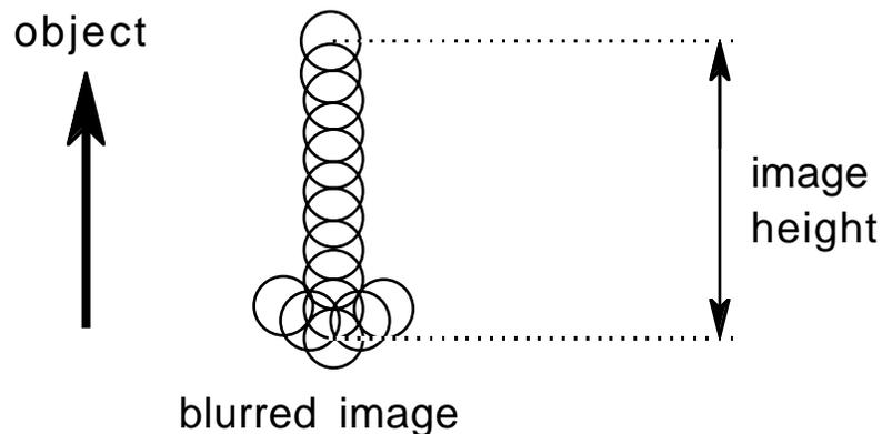
Since the chief ray from a point on the object goes through the center of the blur circle, this is equivalent to saying we measure the distance between the chief rays going to the bottom and the top of the image.
