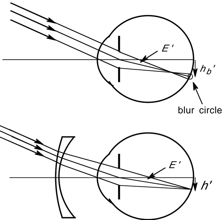
The diagrams above show a myopic eye imaging a remote object. The spectacle magnification in this case would just be  $SM = h'/h_b$ .
