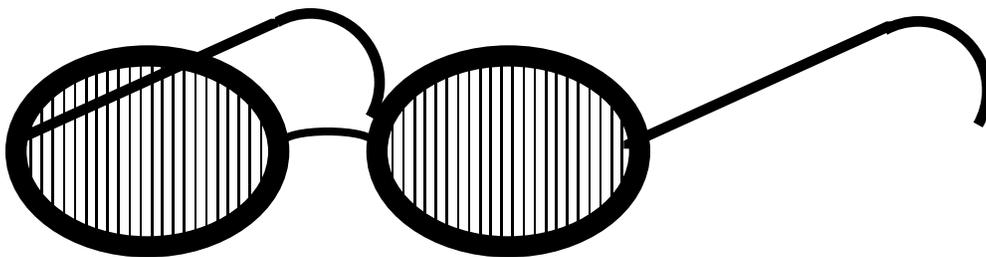
The figure above indicates that polaroid sunglasses contain vertical polarizing filters.
