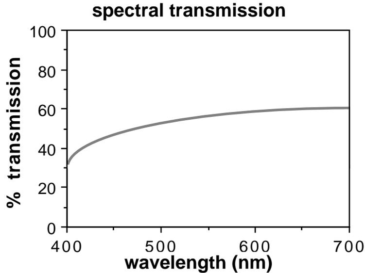
The figure shows the spectral transmission of a typical brown lens. Note the almost linear rise from ultraviolet to infrared.
