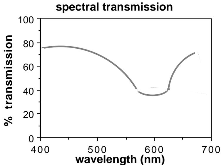
The transmission curves of blue filters show great attenuation of the long wavelengths of visible spectrum.
