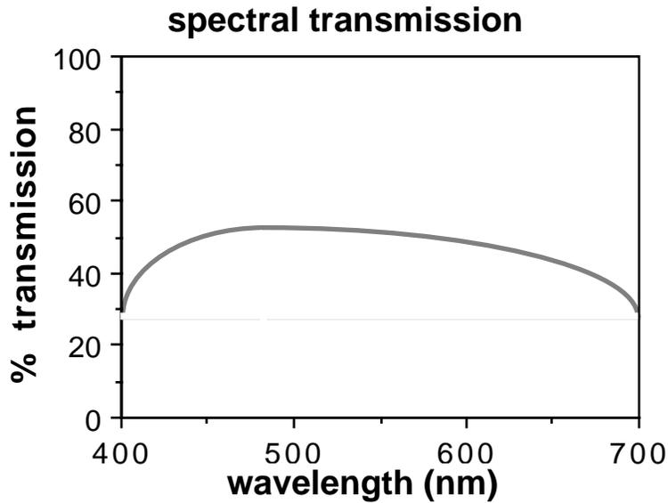
The figure shows the transmission curve of an idealized green tint. Note the peak of the curve shifted towards short wavelengths.
