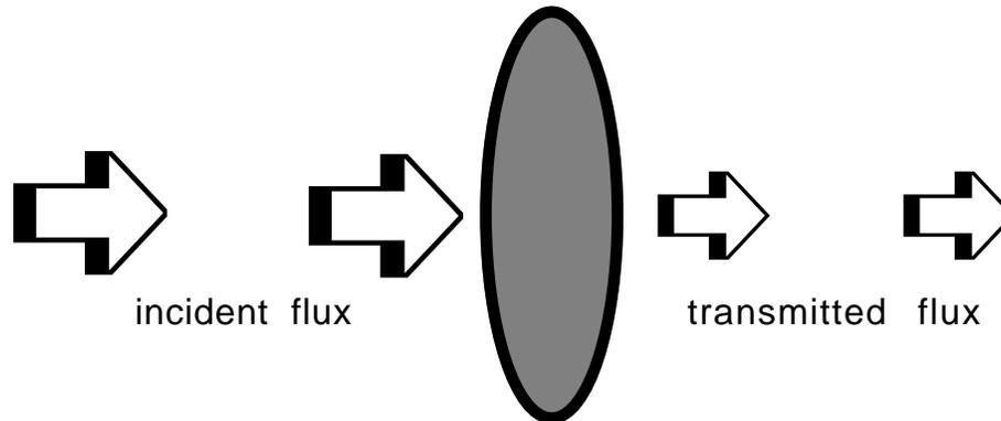
The transmittance or transmission of a lens is the ratio of the light that goes through it to the light incident on it,
