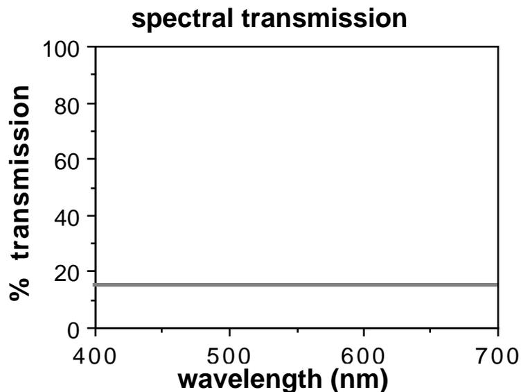
Gray lenses are supposed to be neutral density. The graph above shows an idealized transmission curve for a gray lens. A famous gray tint in glass is the Ray Ban G-15 is a tinted glass with a very flat transmission curve, nearly neutral density in visible spectrum. Its transmittance is 15%.
