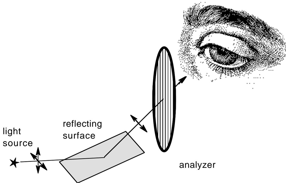
The diagram shows how an unpolarized beam of light is polarized by a reflecting surface such as a road bed or body of water and the now horizontally polarized light is prevented from reaching the eye by the vertically polarized sunglass lenses.
