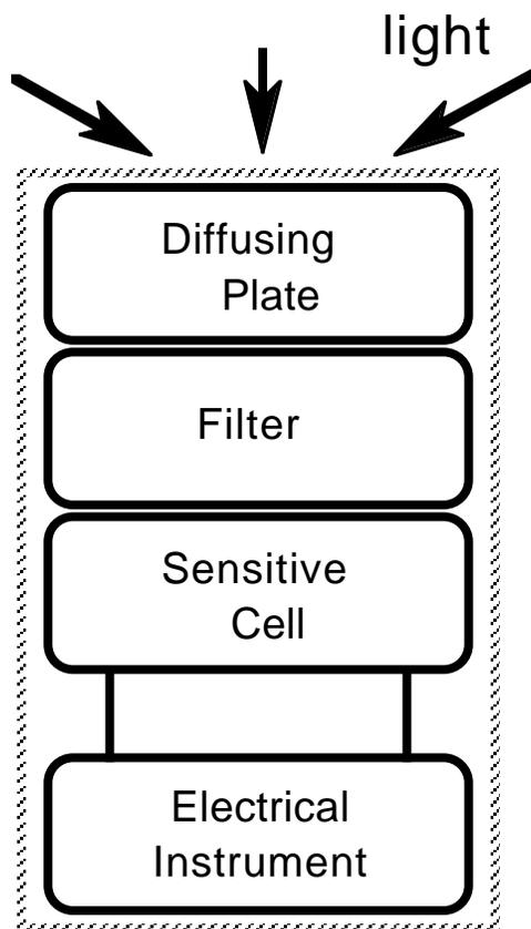
Figure 3. Schematic structure of an illuminance meter.
