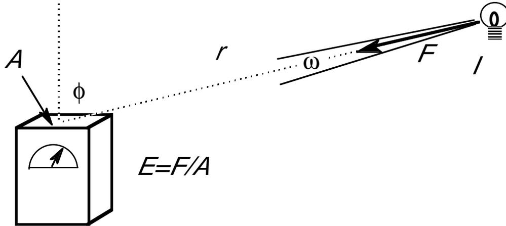
Figure 2. The illuminance of a surface due to a point source of intensity  $I$  is  $E = I \cos \phi / r^2$  where  $r$  is the distance from source to surface and  $\phi$  designates the relative orientation of the surface.
