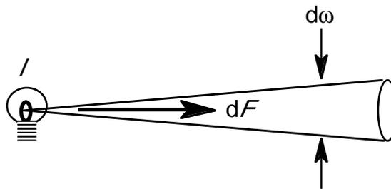
Figure 1. The intensity,  $I$ , of the light filament is  $dF/d\omega$ , where  $dF$  is the flux radiated into solid angle  $d\omega$ . A different value of intensity could result if the solid angle were taken in a different direction since, in general, more flux is radiated in some directions than others.
