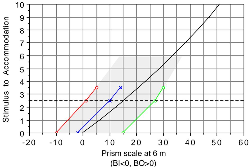
Theoretically the zone of clear single binocular vision should be a parallelogram with its left and right hand sides parallel to the phoria line. In practice there are slight deviations as in the graph.
